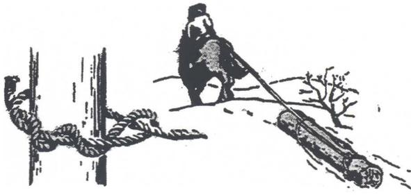
**Timber Hitch** - Used in hauling timber and for commencing the diagonal lashing.
